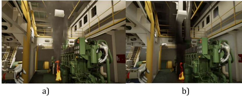
Fig. 10 - Comparison of lower-deck fire visualisation: (a) generic game-engine smoke; (b) CFD-based smoke with airflow deflection
